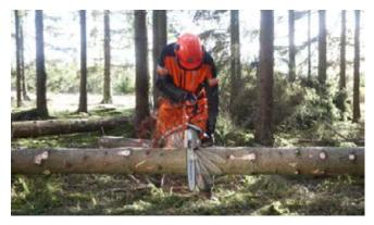
This method is suitable for trees with thin to medium thick branches and regular rounds of branches. For example, if a thick hanging branch is likely to jam the chain and the guide bar, you may need to deviate from the recommended direction of cut on the branches.
