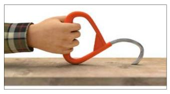
Check the function of the tip by pulling it horizontally, with light pressure on the handle, along the grain on a wooden board or bark-free log. A properly sharpened tip attaches evenly to the wood and ploughs a slight groove.
