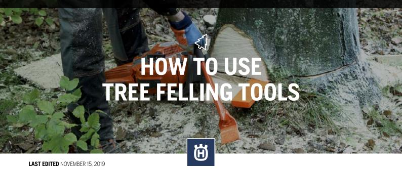
The size of the tree determines which felling tools you need to use. For the smallest trees, you do not normally need the felling tools. Hand force is enough, possibly with a long pole. The felling wedge provides greater felling force than the different types of breaking bar. In extreme cases, you can use a rope and winch, which is the safest and most powerful way to fell a tree.
