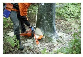
Felling wedges are best for medium to large trees as they provide a lot of lifting force. They are inserted before the felling cut is complete, and are knocked in with an axe or an impact breaking bar. Occasionally, several wedges are needed. It's always good to use wedges made of a soft material, such as plastic or aluminium, should you happen to cut into the wedge, thus eliminating the risk of damaging the chain. Maximum lifting height: approximately 50 – 60 mm.
