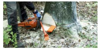
The impact bar is used in the same applications as the breaking bar. It can also be used as a striking tool when using felling wedges.
