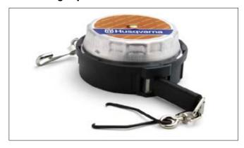
The most common logger tape is 50 feet/15m long, but it's available in many other lengths. The tape should be equipped with a swivel snap for attaching it to a belt as well as a quick-release nail end that you attach to log ends, making it easy to move the needed distance, along the tree or log, to measure length or diameter correctly, then release the nail with an easy tug.
