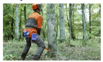
The breaking bar is available in different handle lengths providing you with varying amounts of felling force. Avoid breaking bars with a long handle for really thick trees and large backward leans, as this may require a lifting height that is greater than you can handle. Maximum lifting height: approximately 2 cm.
