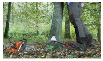
The foot breaking bar is suitable when thinning and for smaller trees. Insert the foot breaking bar before completing the felling cut. Stand and put all your weight on the lever arm. The foot breaking bar is generally telescopic and can be carried in a holster on your logging belt.
