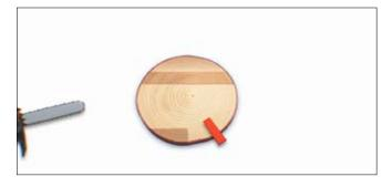
Insert the wedge or breaking bar.
