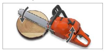
You can also saw from the opposite direction using a pushing chain and apply the upper tip of the bumper spike. However, sawing this way usually becomes more irregular and there is greater engine resistance.
