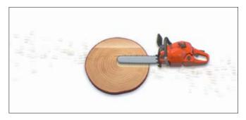
Make a bore cut to about 60 % of the tree diameter.
