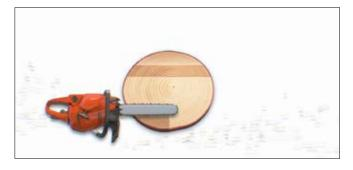
Change your position to the other side of the tree. Make a bore at 60% of the tree diameter and cut straight backward until you have shaped a suitable corner.
