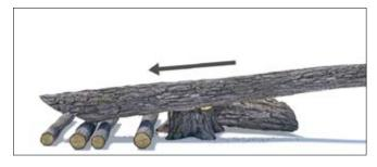
Performed correctly this is the result of the step down method. The tree splits from the stump, slides backwards on the sliding surface, releases from the tree it got hung-up on and falls to the ground.
