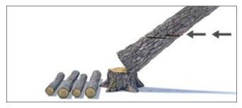
Knock in the wedge until the wood fibres split between the two cuts. Stay alert – the trunk usually slides off the stump at the same time.
