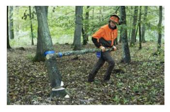
Take the turning hook (or use the turning strap to attach a branch as a lever) and roll the tree away from you. Lift straight with a straight back and knees bent. If the tree is large or has hung really tightly, you can increase the rolling force by using the turning hook or turning strap with a longer piece from a thin tree.
