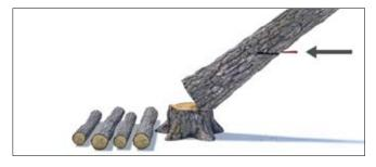
Insert a wedge to prevent the backside cut from pinching.
