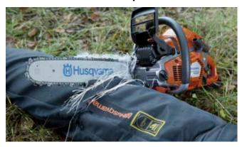
Protective trousers must be fitted with saw protection that meets international standards. The saw protection consists of a lining with several layers of very long fibres that become entangled in
