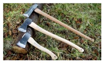
Use an axe to remove bark, soil and sand from the log before cutting, as this will reduce wear on the guide bar and chain. You also use the axe to knock in the felling wedges.
