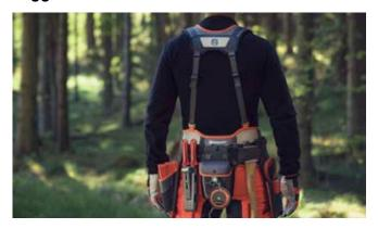
A complete tool belt for a professional logger. Flexible for different tools like lifting hooks/tongs, wedges, axe, measuring tape, files and first aid kit.
