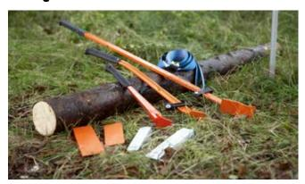
You should always include breaking bars and wedges of different sizes when felling trees. As well as a turning strap if you accidentally fell a tree against another tree. A hand winch is also useful to have to bring down a hung tree. For particularly difficult or sensitive felling, you should also include a winch, rope and pulley as well as a means for attaching a rope high up in a tree if needed. Read more about felling tools on chainsawacademy. husqvarna.com
