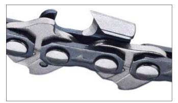
If you are used to filing, you can also file without the filing gauge. Be sure to maintain the original angles for the cutting teeth. To maintain the correct angle and depth of the cutting teeth, we recommend that you keep on using the filing gauge even after you've filed freehand a few times.
