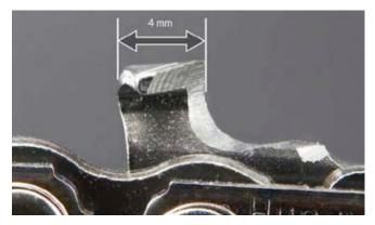
It's time to replace the chain when the longest portion of the cutting tooth has been worn down to less than 4 mm, or if you find cracks.
