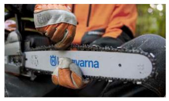
Make sure the chain is correctly tensioned. A slack chain can jump off the guide bar, cause injuries and damage the chainsaw. A slack chain – as well as an overly tight one – can also cause premature wear on the bar.
