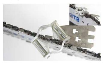
**FILE WITH BOTH HANDS** Place the file at a 90-degree angle in relation to the rollers on the filing gauge. The file should rest on both rollers. The filing angle is then 25–35 degrees depending on the type of chain. File the cutting tooth away from you, with smooth strokes.
